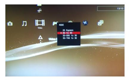
4. When you connect first, the default mode is "Bypass Mode". You can watch TV as usual (without the glasses) and the LEDs will look like this:
