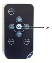
This will show the current HDMI source that is selected, the mode of operation and the input and output resolutions of the converter box.
